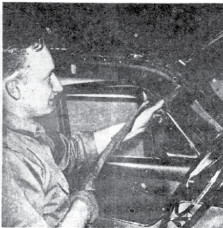
4. Remove kick panels for further access to windlacing. Then with headliner retaining strip over door removed, windlacing can be taken off.
